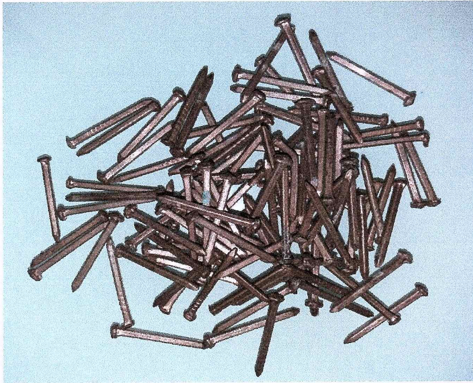
Copper nails used as positive conductor
