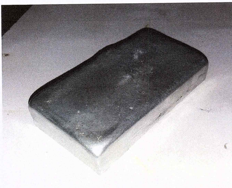
Pure zinc used as a negative conductor
