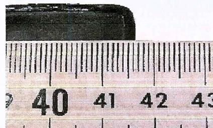
**Figure 2.** An example of a meterstick reading. The object length is measured to be 41.64 cm.
